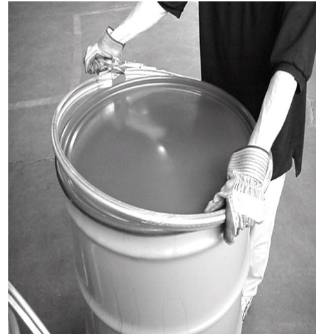
Figure 7 – Expanded ring being placed on drum
